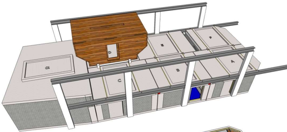
3D illustration of the acoustic laboratory, showing the overhead crane, the mobile room M and the ceiling slabs with local savings (rooms illustrated without doors).
