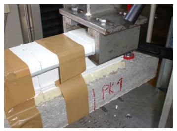
**Fig. 7** Test set-up for tensile test
