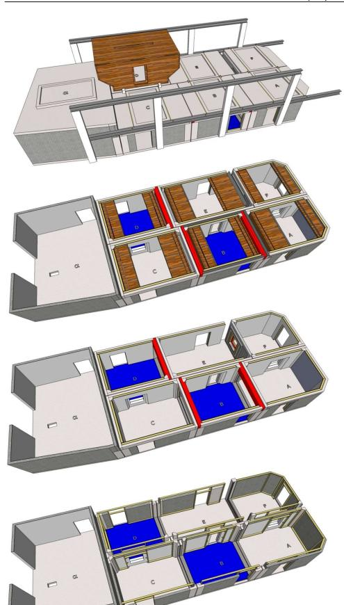
3D illustration of the acoustic laboratory, showing the overhead crane, the mobile room M and the ceiling slabs with local savings (rooms illustrated without doors).
